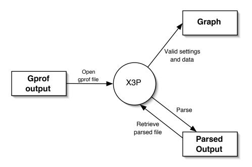
Explanation: The initial data is in the form of unparsed gprof output. The user can open it and let our system operate on it. The system will then parse the raw gprof file and create a file recognizable by our system. The system will use that data to create the graph.
